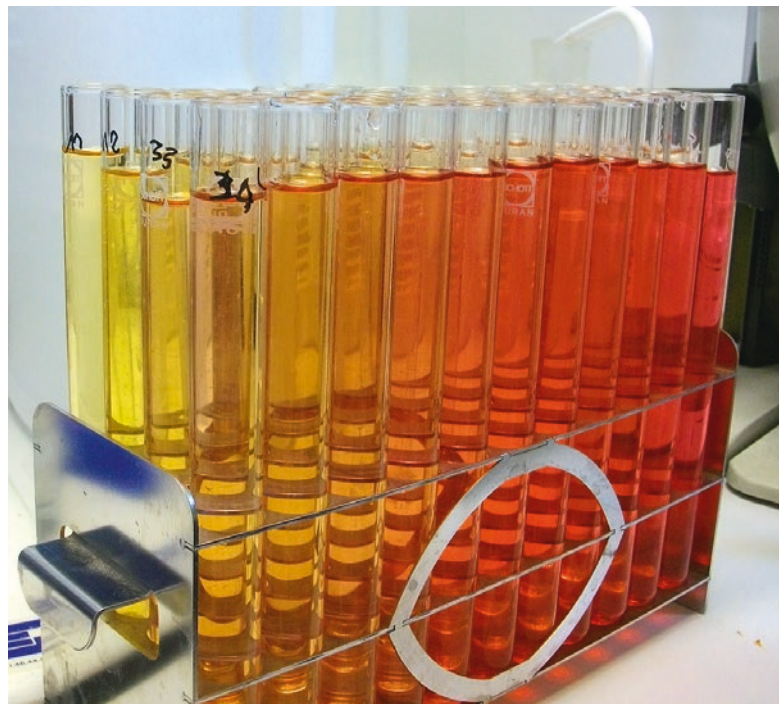
▲ Separation of phenolic compounds of wine, with yellow staining due to tannin oxidation
