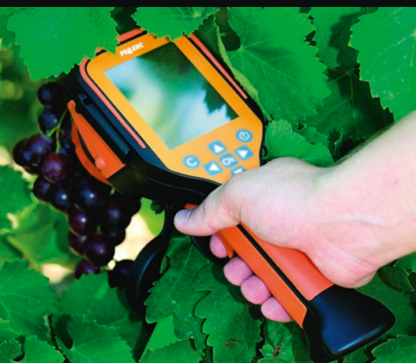
▲ Spectron™, a portable sensor for monitoring grape ripening © Pellenc SA
