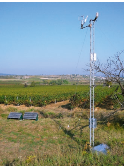
▲ Evapotranspiration measurement device set up in the Roujan catchment © L. Prévot/UMR LISAH
